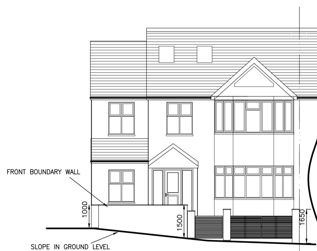
EXISTING FRONT ELEVATION WITH FRONT BOUNDARY WALL 1:100
