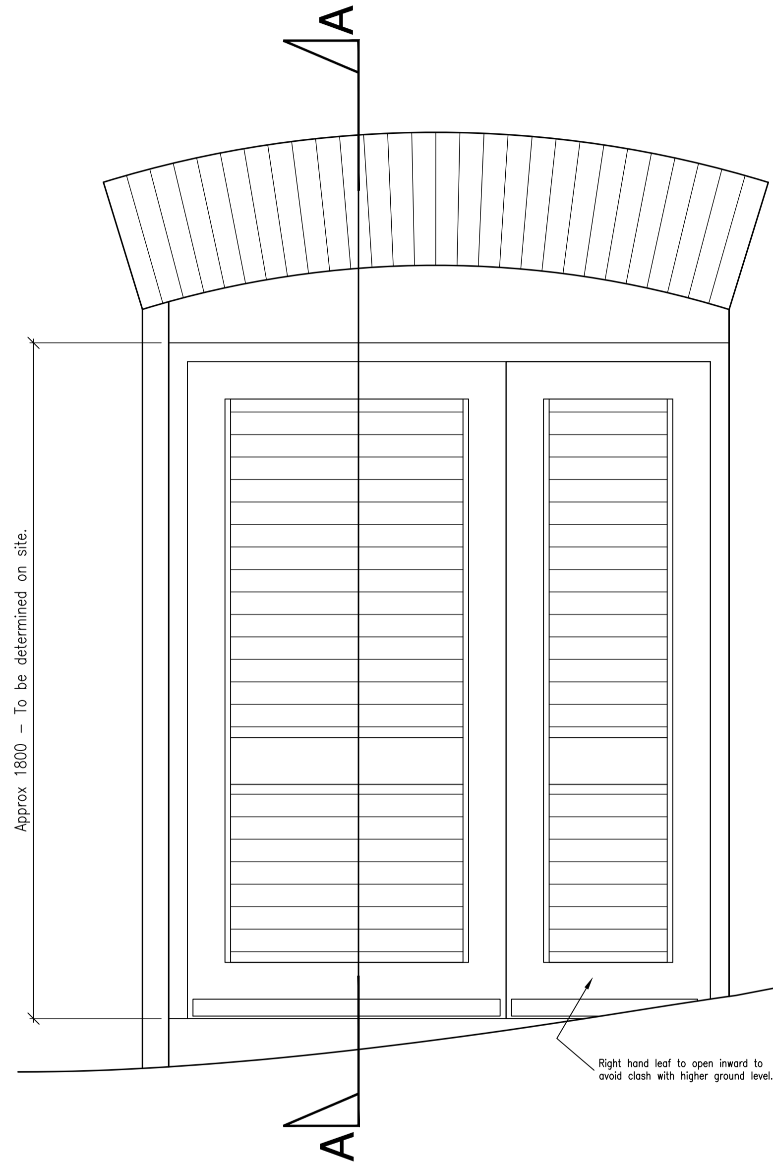
Sub-Station Door - ED04 Hardwood door and frame with white painted finish.
