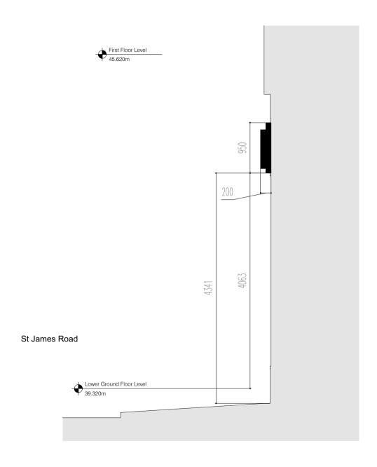
All sign panels formed from folded composite aluminium trays with 100mm returns. Letters are proposed in built up 100mm acrylic, internally illuminated with low energy LED lights.
