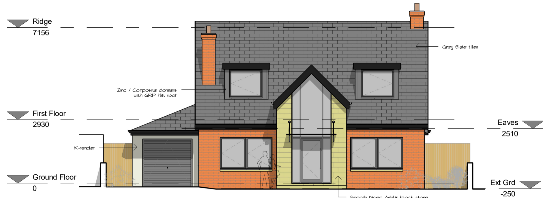
Front Elevation (East Facing) 1 : 100
