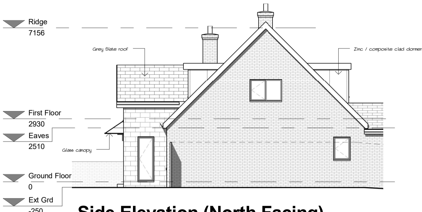
Side Elevation (North Facing) 1 : 100
