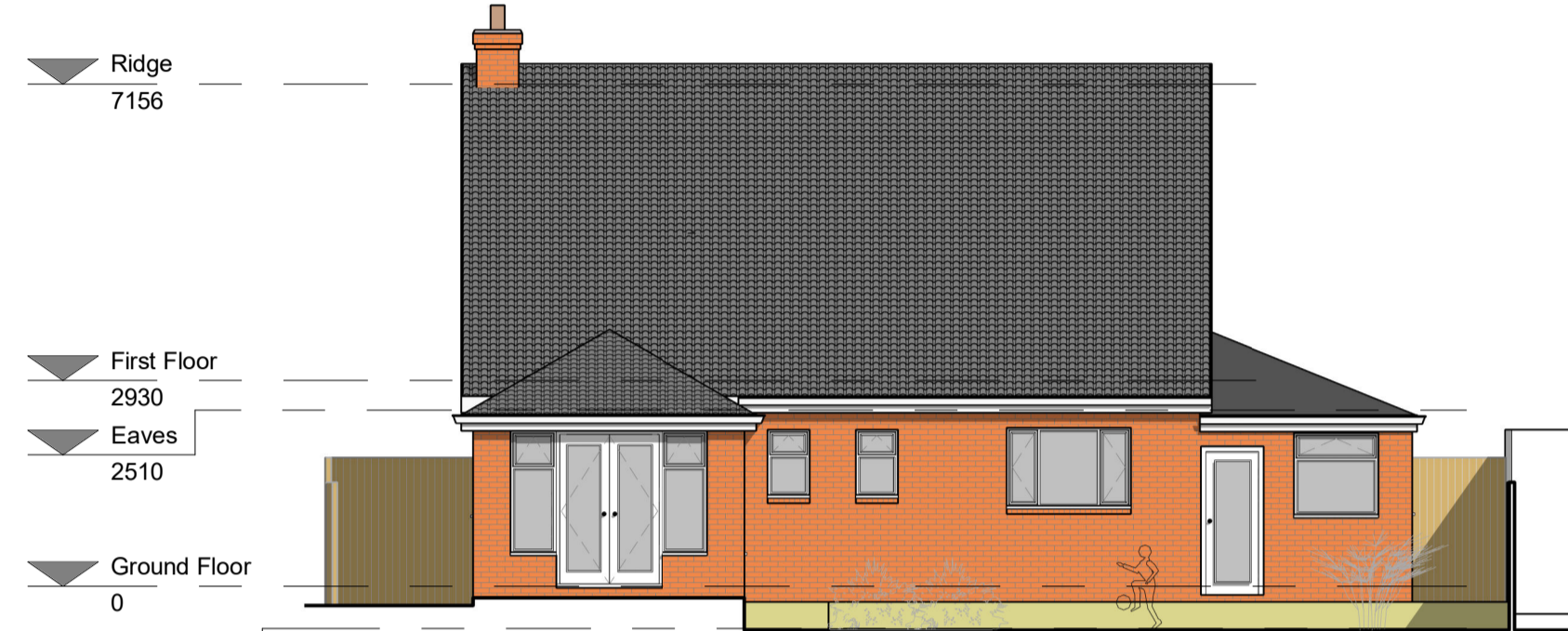
Rear Elevation (West Facing) 1 : 100
