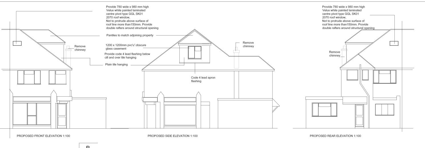
В 5684 mm 350 x 20 x 100 350 x 20 x 100 bearing plate bearing plate 1340 mm Α 3895 mm  $\boxtimes$ 1800 mm Remove chimney 350 x 20 x 100 350 x 20 x 100 bearing plate bearing plate PROPOSED LOFT PLAN 1:50 В ELECTRICAL: All electrical works are required to meet the requirements of Part P (ELECTRICAL SAFETY) must be designed, installed, inspected and tested by a person competent to do so.
