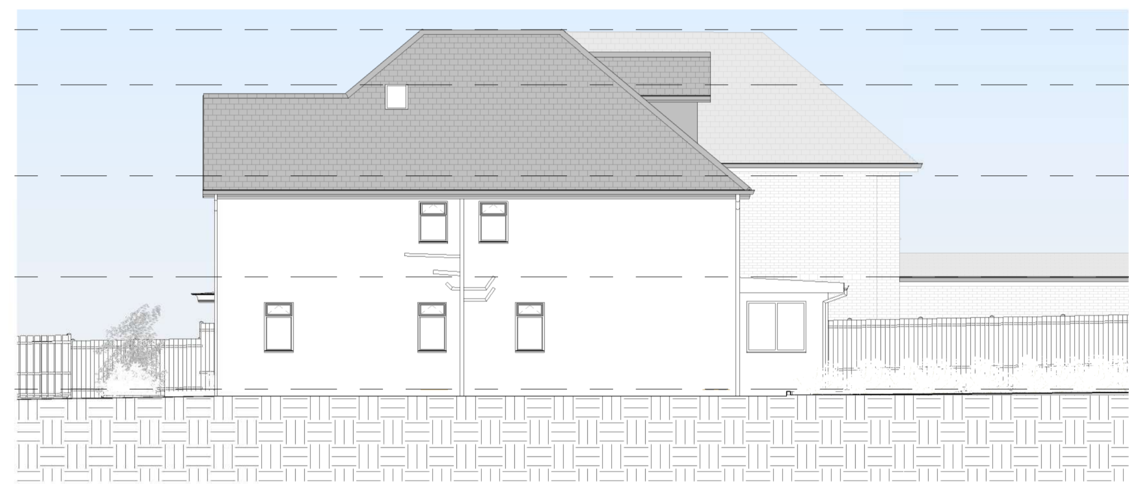
4 Existing Right Elevation 1 : 100
