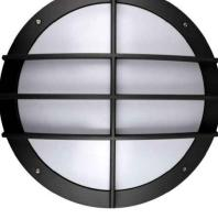
L2 PROPOSED SIDE ACCESS LIGHTING TO BE THE KOSNIC CIRCULAR CAST ALUMINIUM BULKHEAD GRILLE IN BLACK IP65 WITH OPAL DIFFUSER OR SIMILAR WITH DUST TILL DAWN SENSOR AND OVERRIDE SWTICH BACK TO LANDLORDS POWER SUPPLY. DIMENSIONS ARE 363mm DIA. AND 172mm DEEP. LED COMPATIBLE.
