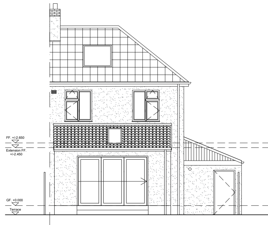
EXISTING REAR ELEVATION (A)
