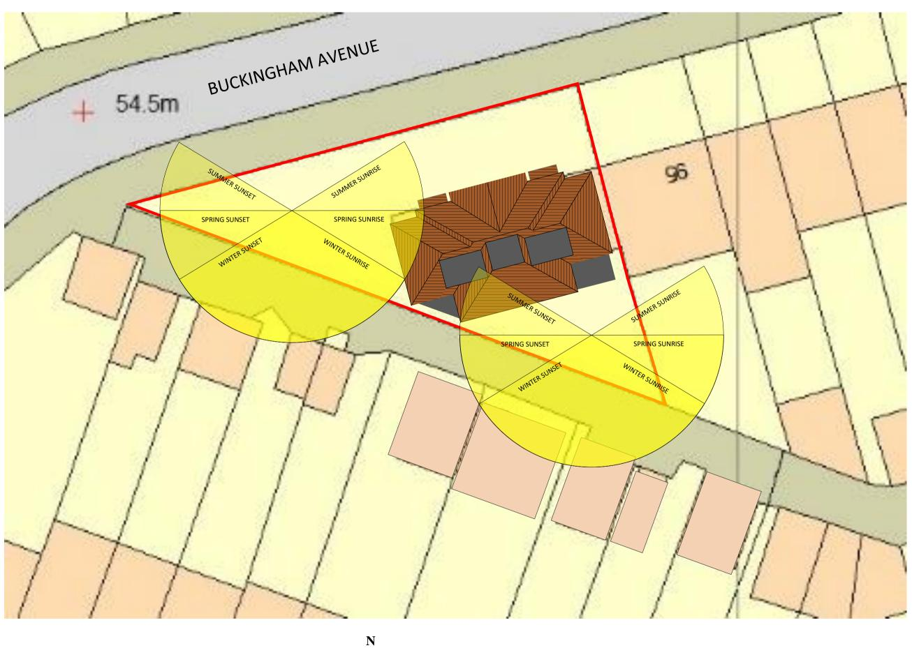
95aBAW 526 – PROPOSED BLOCK SITE PLAN – LOFT FLOOR 95a BUCKINGHAM AVENUE, WELLING DA16 2ND SCALE 1: 200 PRINTED ON A3 USING MS WORD OR PDF
