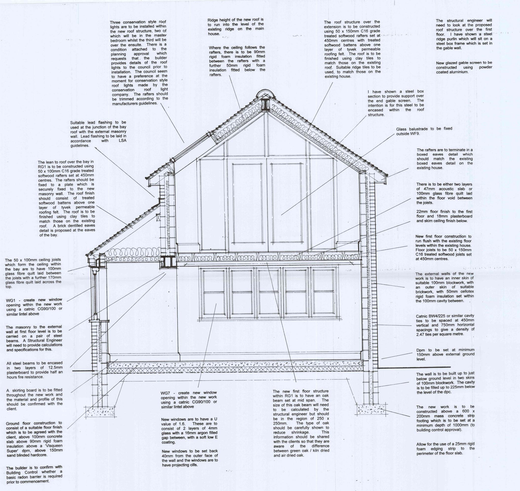
New guttering to match the profile used on the existing house, unless the clients specify that all of the existing guttering is to be renewed.
