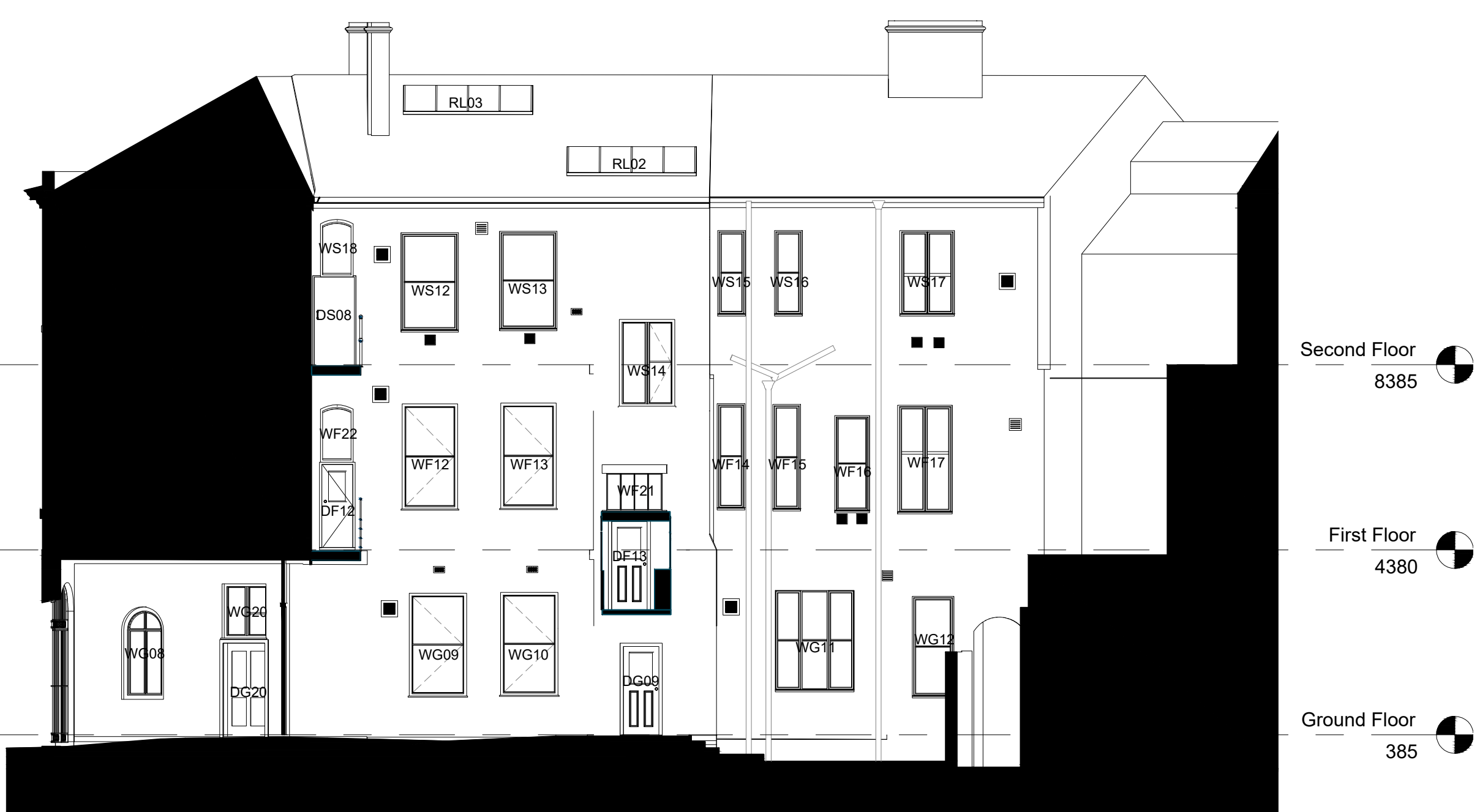
3 1030 Rear Courtyard - West Elevation as Existing 1 : 100
