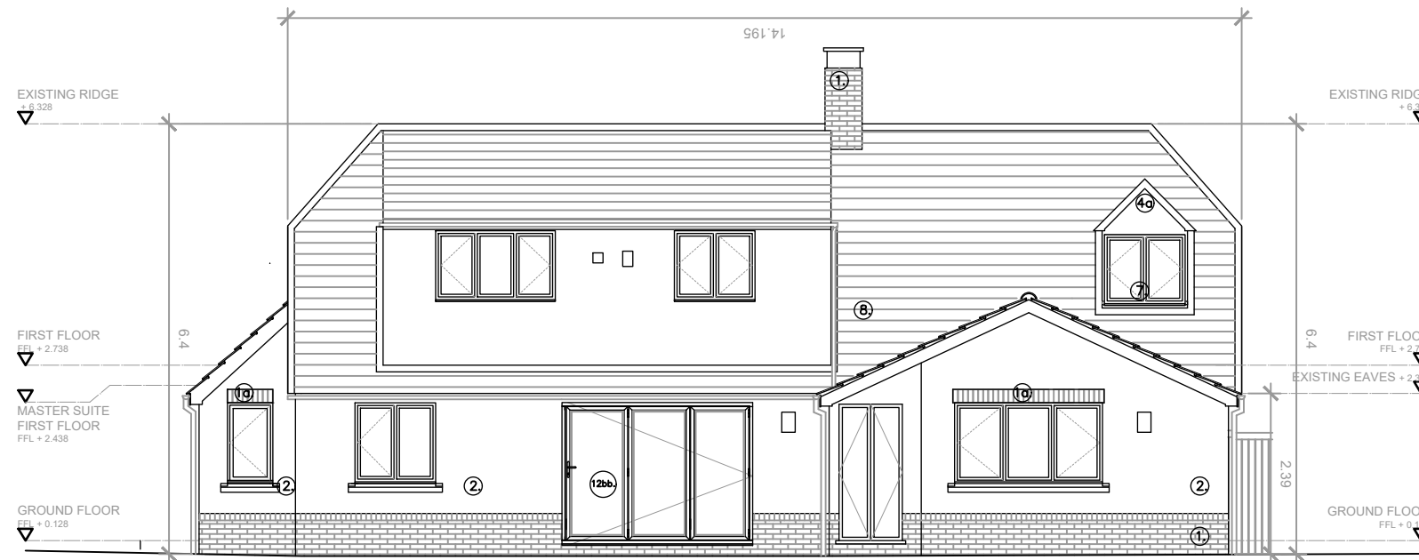
3.) PROPOSED REAR ELEVATION C-C (Datum 43.00m)
