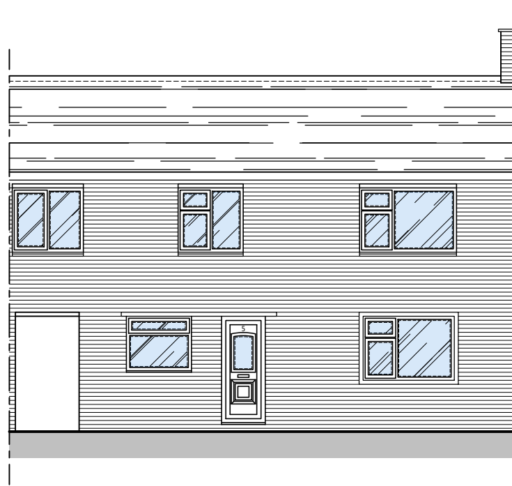
EXISTING FRONT ELEVATION SCALE 1:100
