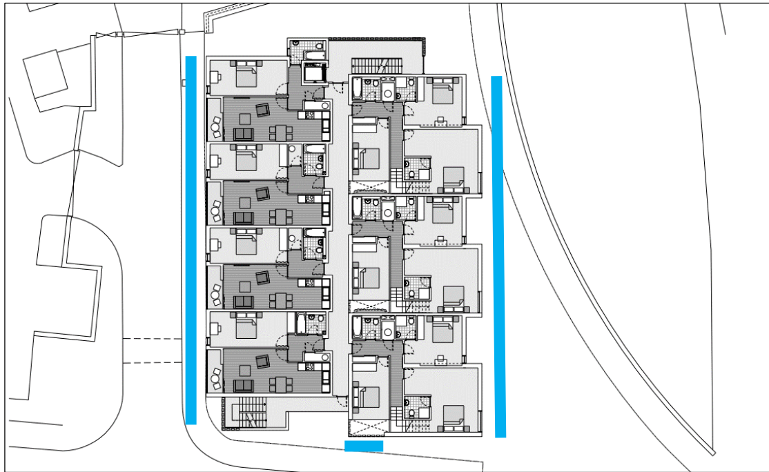
Proposed façade zones for controlling entertainment noise.
