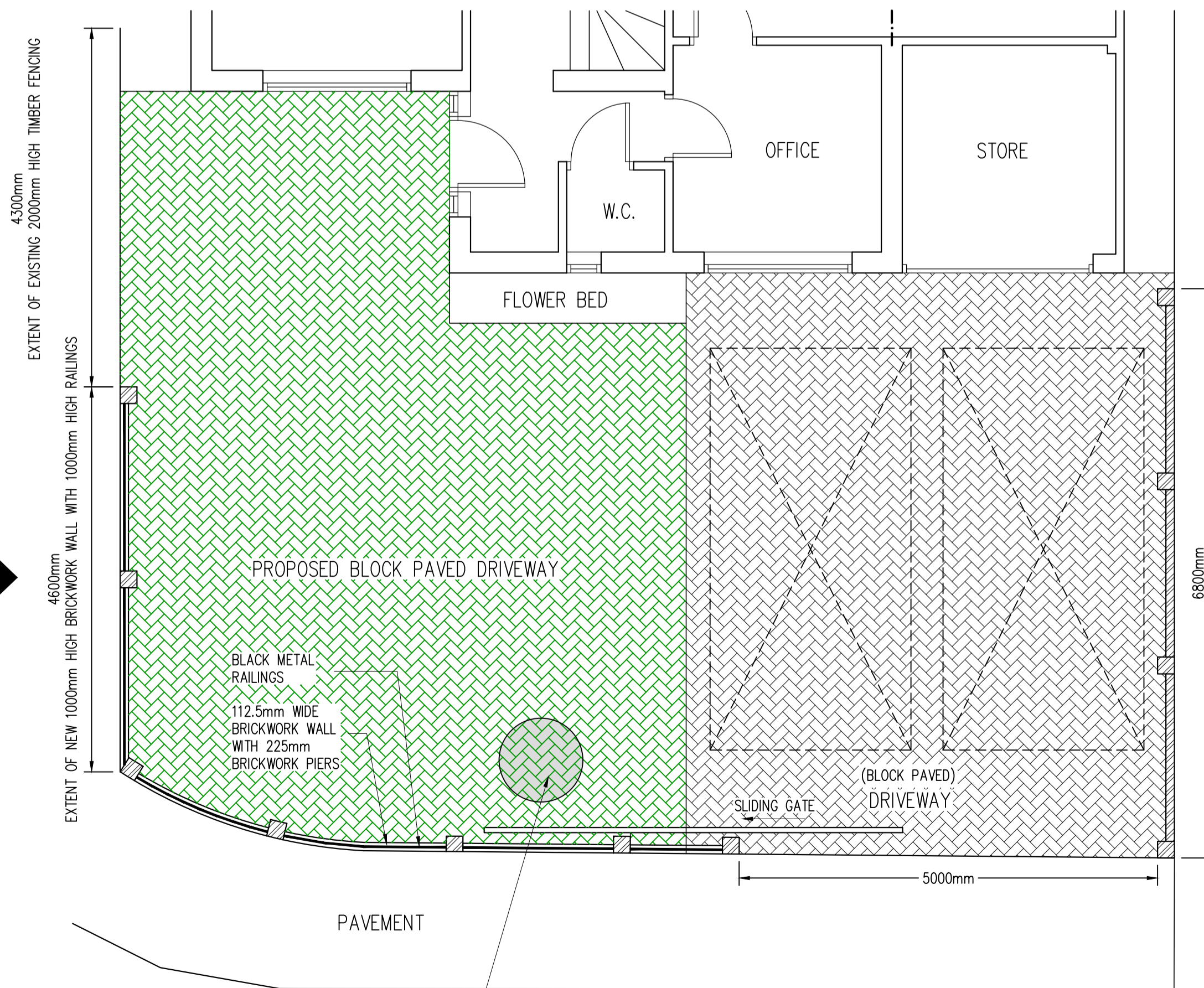
(HOWELLS CLOSE) PROPOSED SITE PLAN SCALE 1:50
