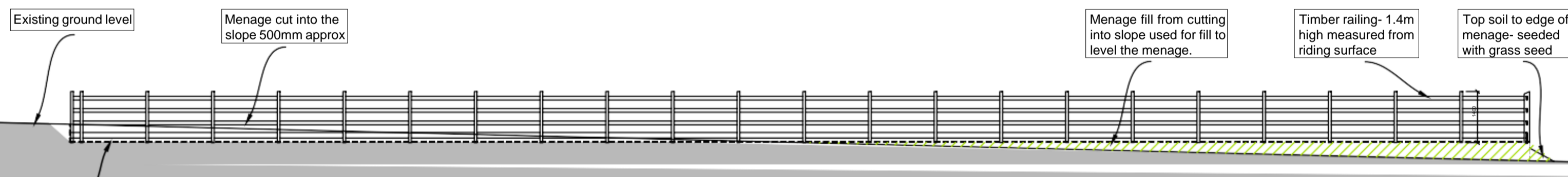
Proposed menage surface level - dashed line SECTION E-E THROUGH MENAGE 1:100
