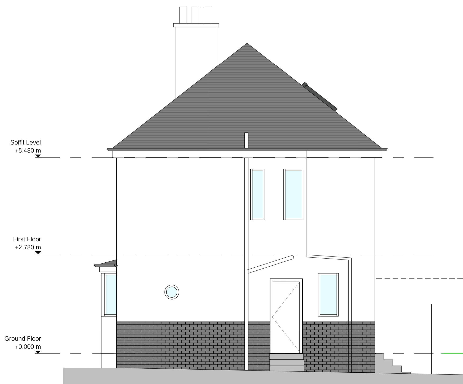
Existing Side Elevation 1 : 50
