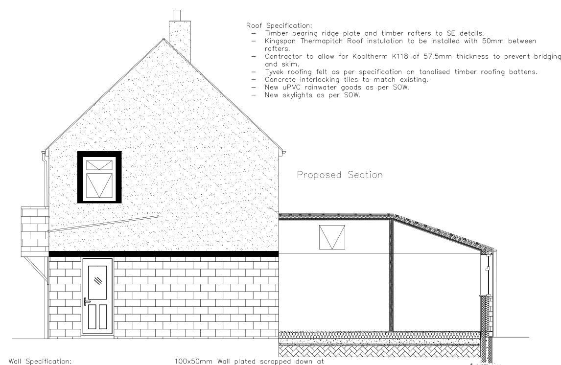
New cavity external wall a top strip foundation from inner leave 100mm aerated 7.3 KN blockwork and external leave coursed New Permaguard 500-micron DPC or equal stone work to match existing.
