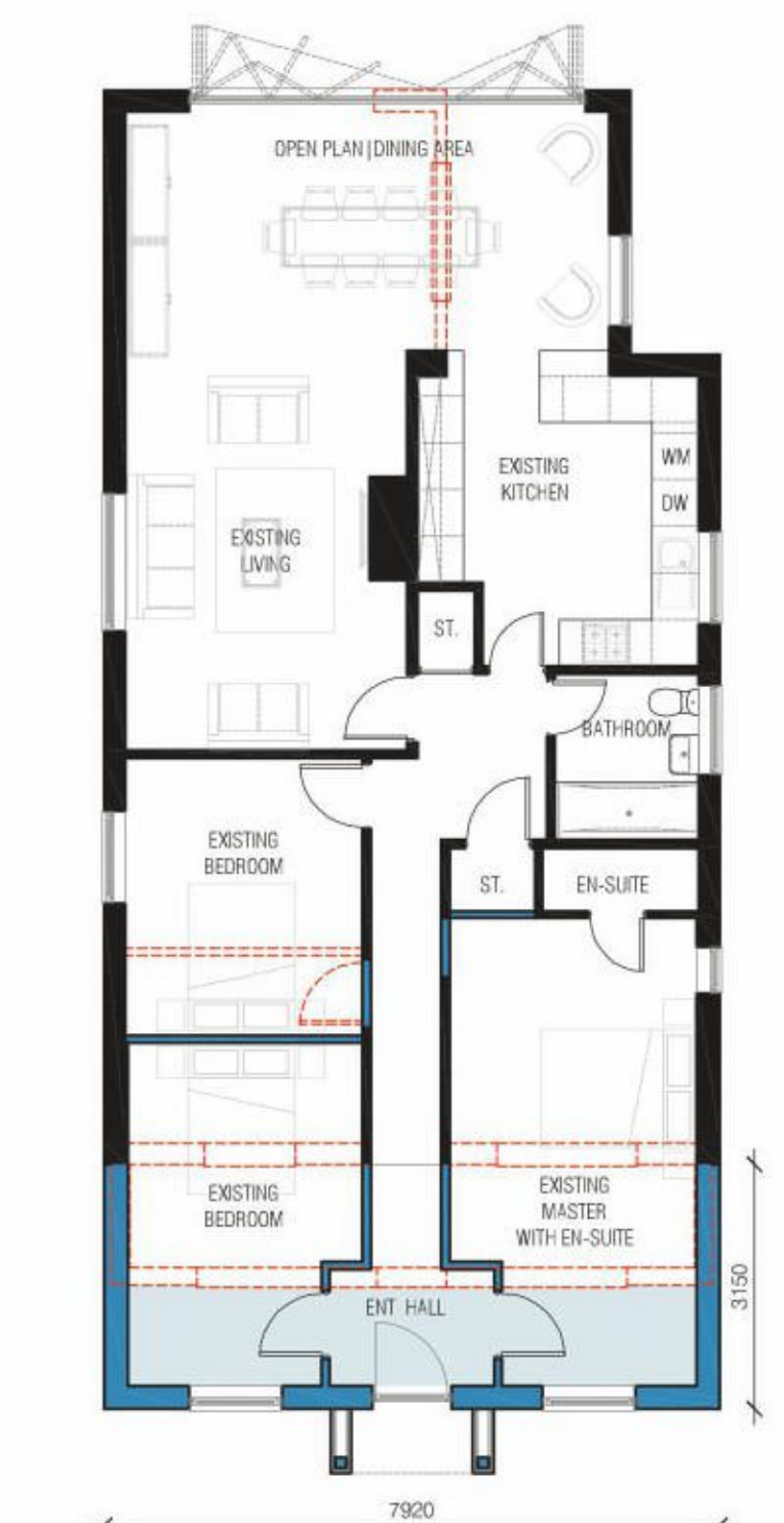
PROPOSED FLOOR PLAN SCALE: 1:100@A1
