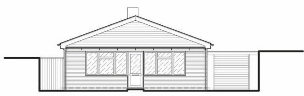
EXISTING FRONT ELEVATION SCALE: 1:100@A1
