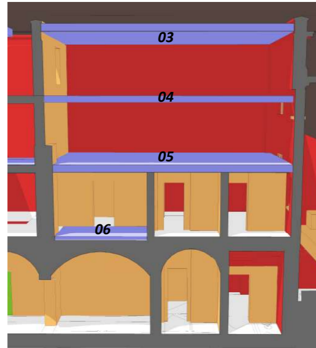
New floor levels added
