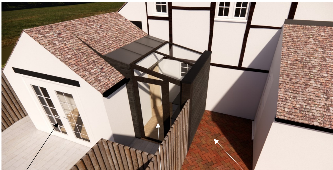
New patio door and timber lintel above
