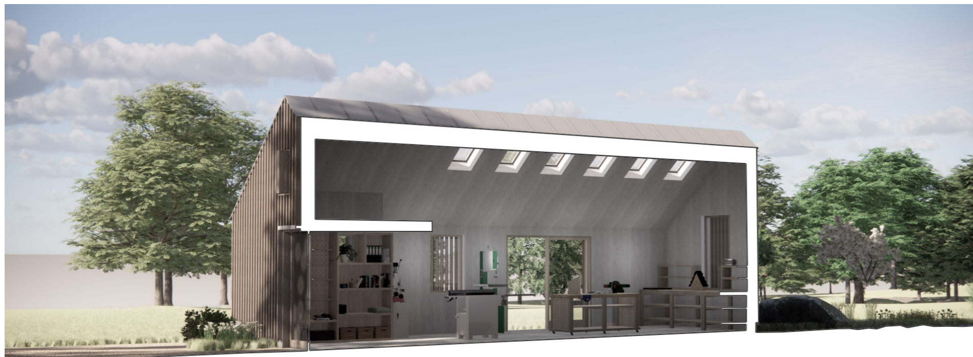
Fig.45 _ Section through Workshop showing overhead storage area
