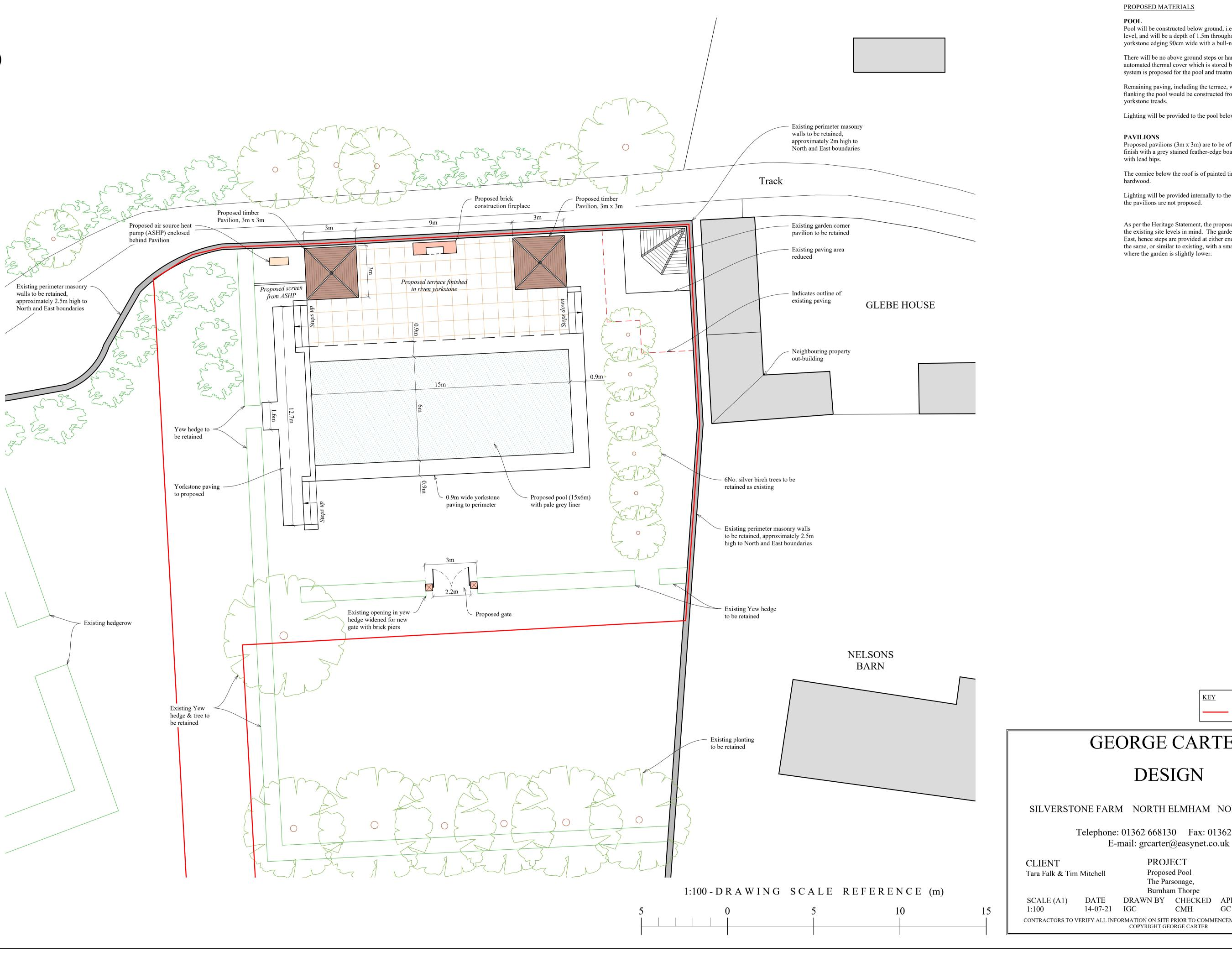
Pool will be constructed below ground, i.e. not raised above existing garden level, and will be a depth of 1.5m throughout. Pool will have a grey liner with cut yorkstone edging 90cm wide with a bull-nosed edge to pool.
