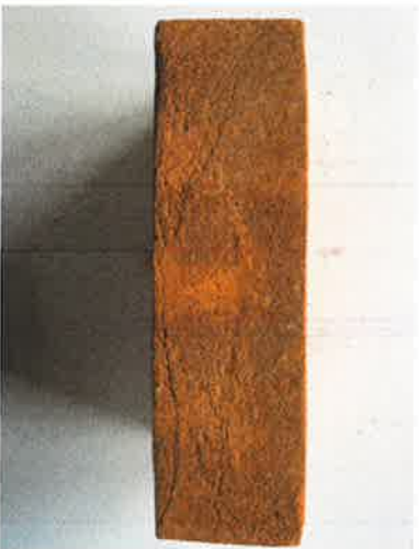
21/00456/LBCALT | Condition 6 21/02110/DETAIL Walls - Imperial red rubbers [mixed with glazed snapped headers] by Lambas with Lime Mortar bond to match adjacent
