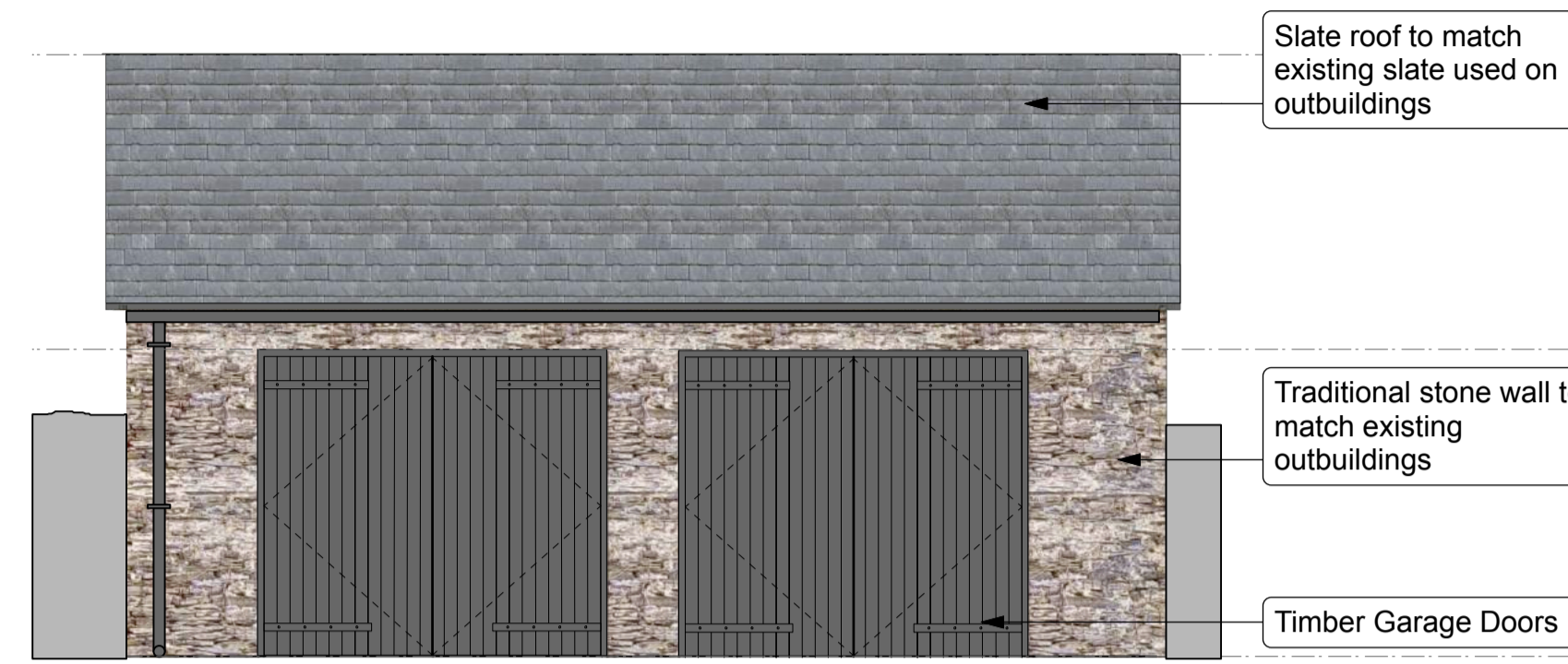
2 Garage Front Elevation SE Facing Scale: 1:50
