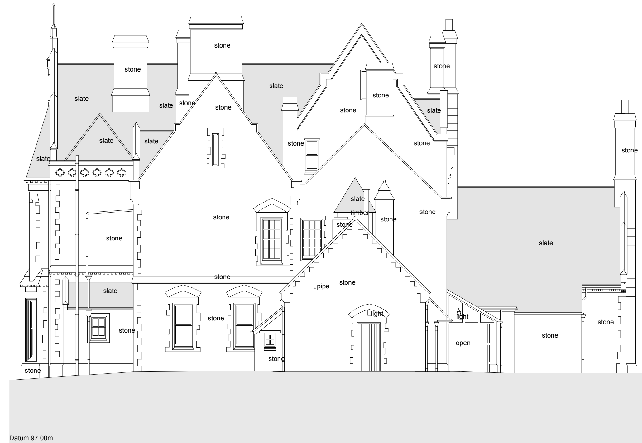
Datum 97.00m NORTH WEST ELEVATION
