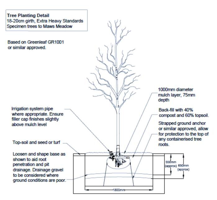
\*Note - Dimensions for tree pits to be agreed with the site supervisor, in line with Table 30/1, 3000 series, DMRB Volume 1.
