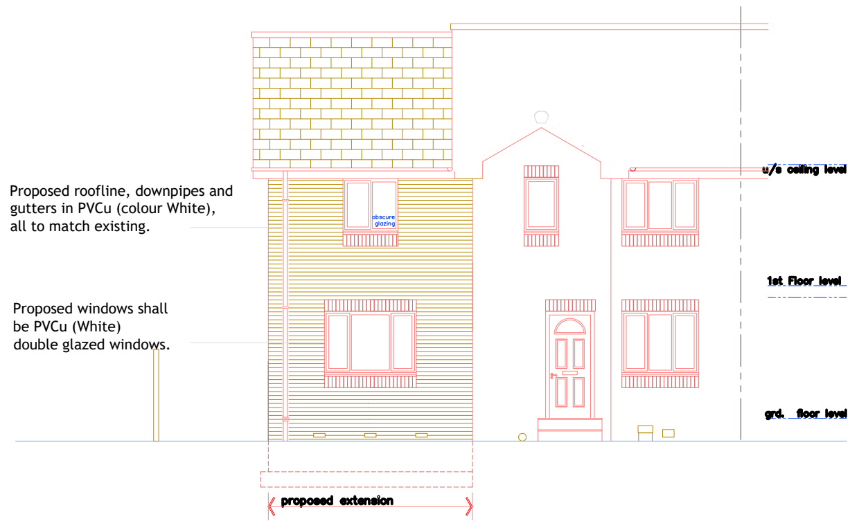
Proposed North Elevation scale 1:100
