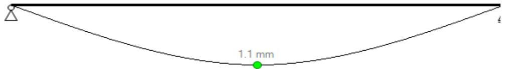
Loadcase: 5 Imposed Major Deflection for TR Base/A/1-Base/F/1
