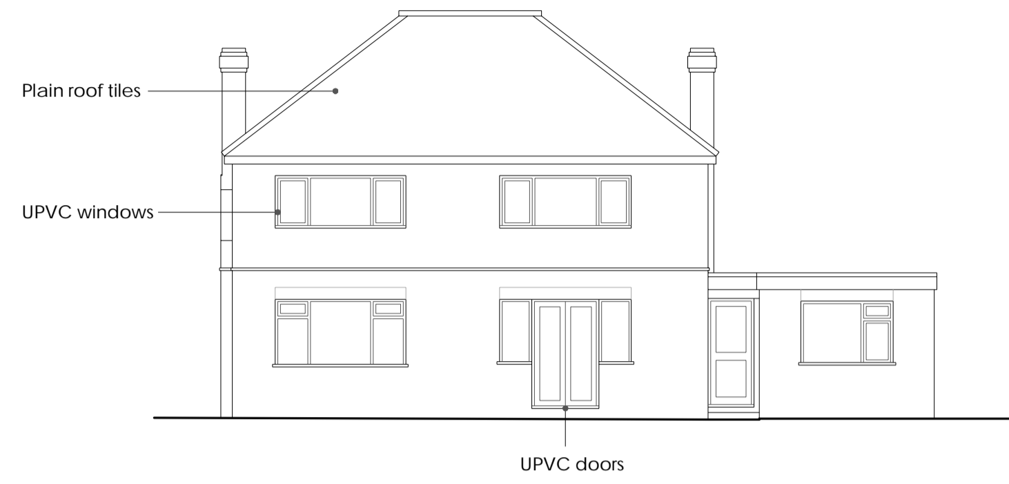
Rear Elevation As Existing
