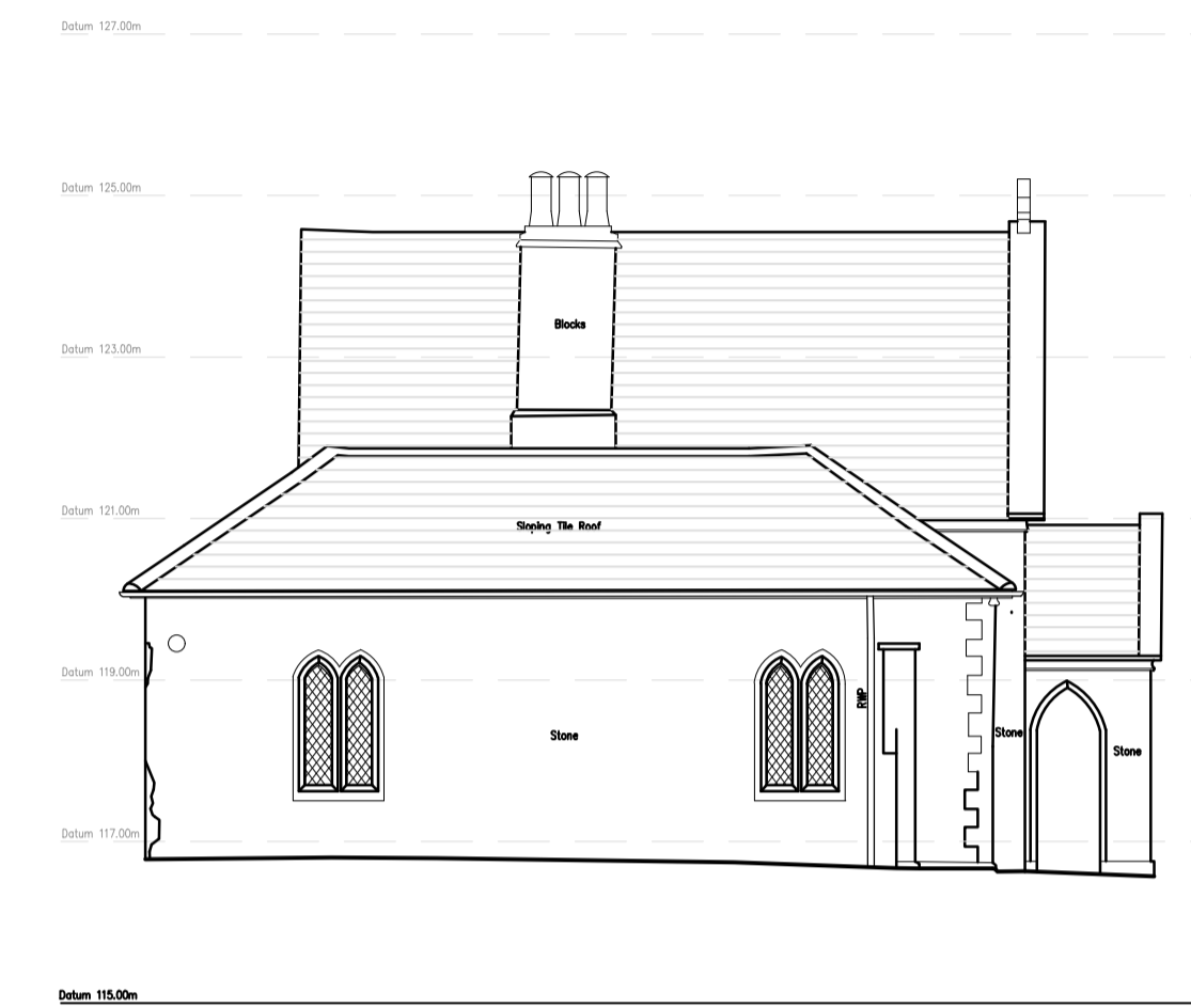
EXISTING SIDE (NORTH WEST) ELEVATION
