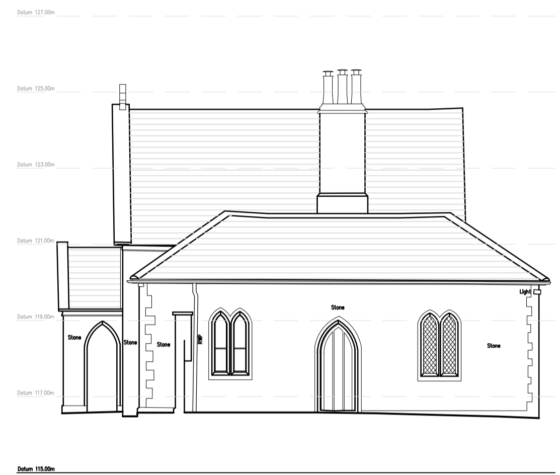
EXISTING SIDE (SOUTH EAST) ELEVATION
