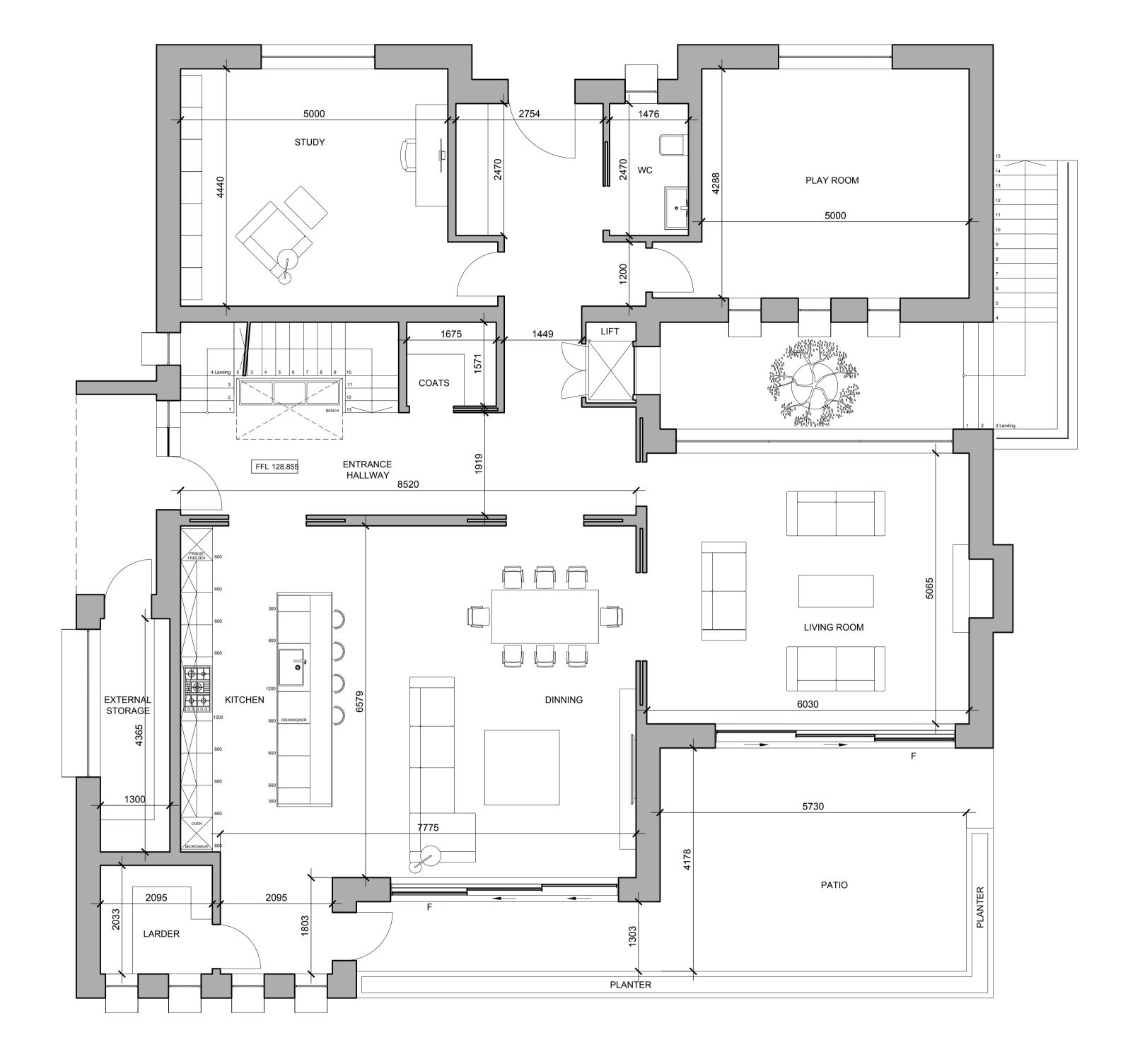
PROPOSED UPPER GROUND FLOOR PLAN SCALE 1: 50 Figured dimensions only are to be taken from this drawing. All dimensions are in millimeters unless otherwise stated. All dimensions shall be checked on site prior to works
