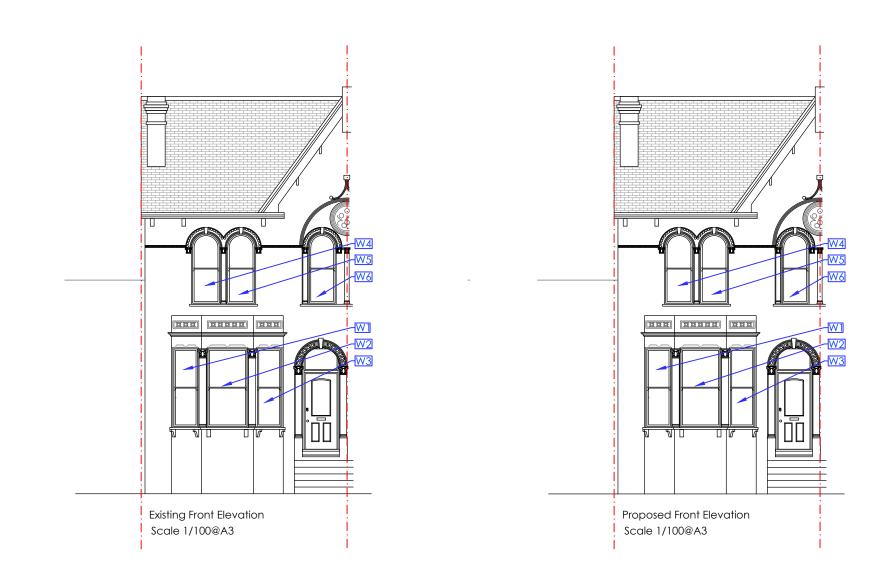
W1,W2,W3 - New double glazed box timber sash windows , painted white W4,W5,W6 - New double glazed timber sashes into the existing box frames, painted white
