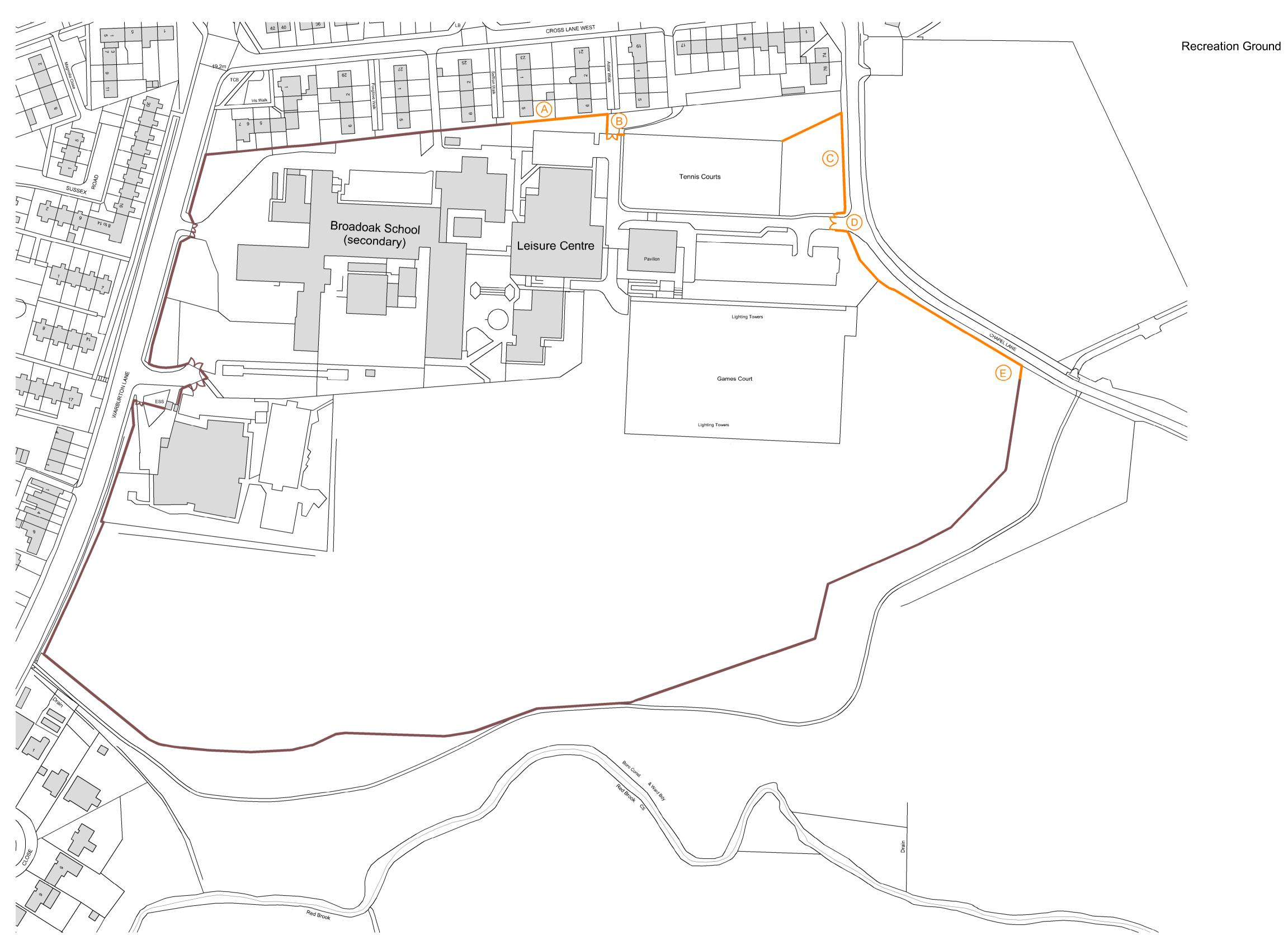
Orange line indicates new fence & gate 2.4m high 358 Weldmesh PPC Green, RAL 6005
