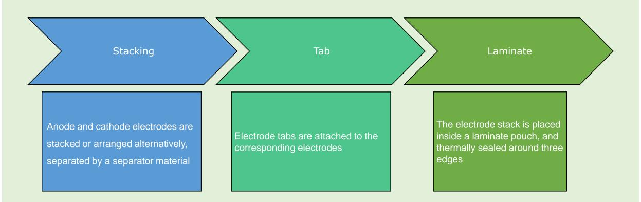
\*Cell Production is completed in a clean, dry environment to prevent moisture interaction with cell components and particulate contamination
