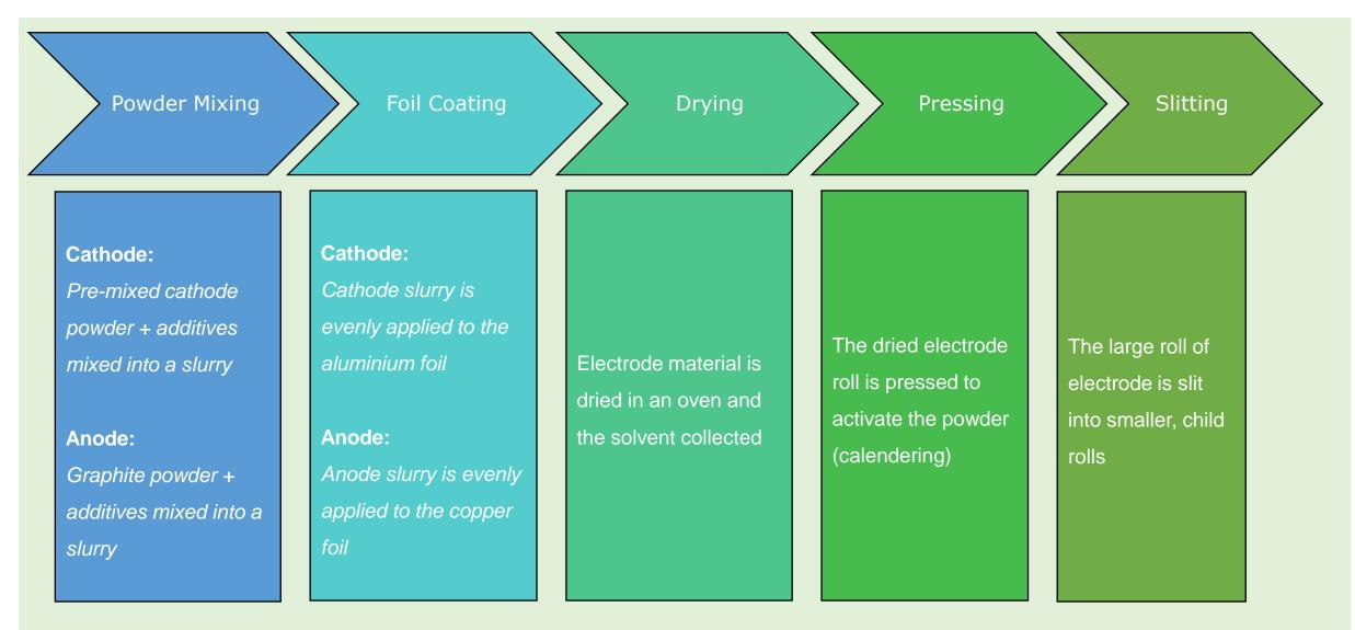
\*Cathode and anode electrode manufacturing is completed in separate environments to prevent cross-contamination
