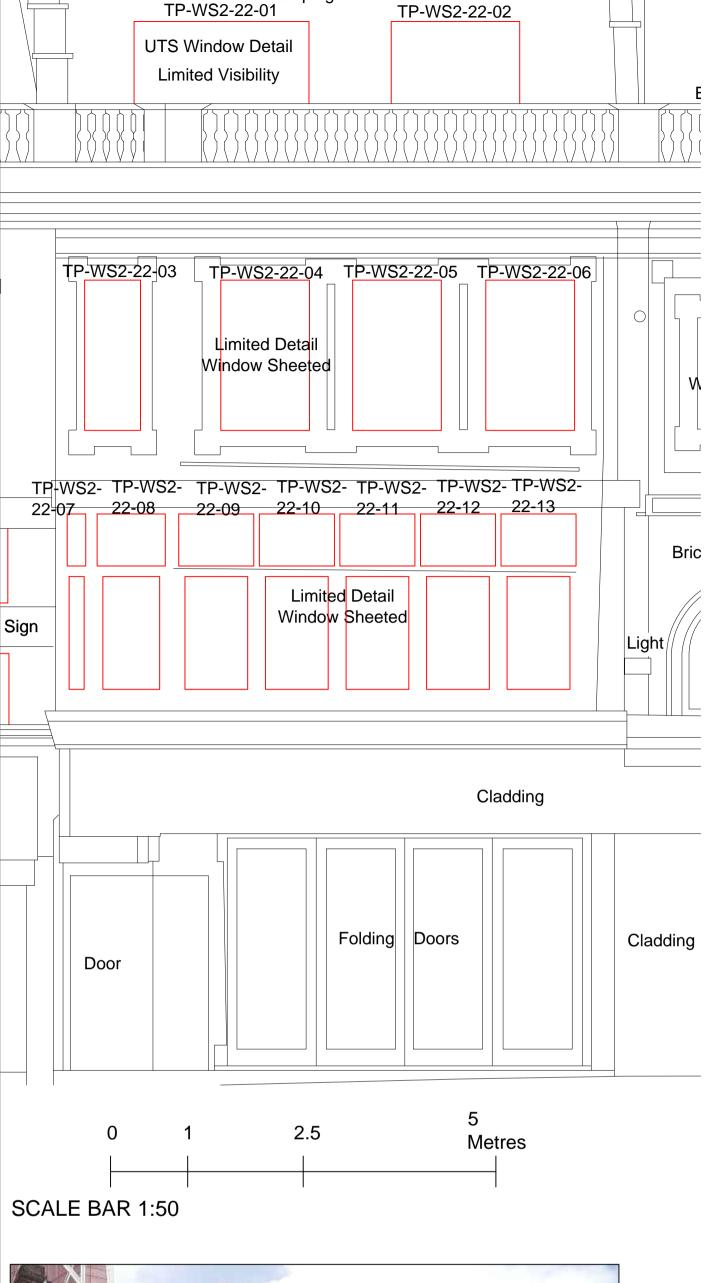
1:50 elevation drawing, showing sample portion of existing casement windows, located on Terminus Place.
