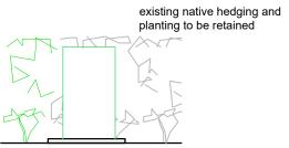
new 700L bunded oil tank on concrete base
