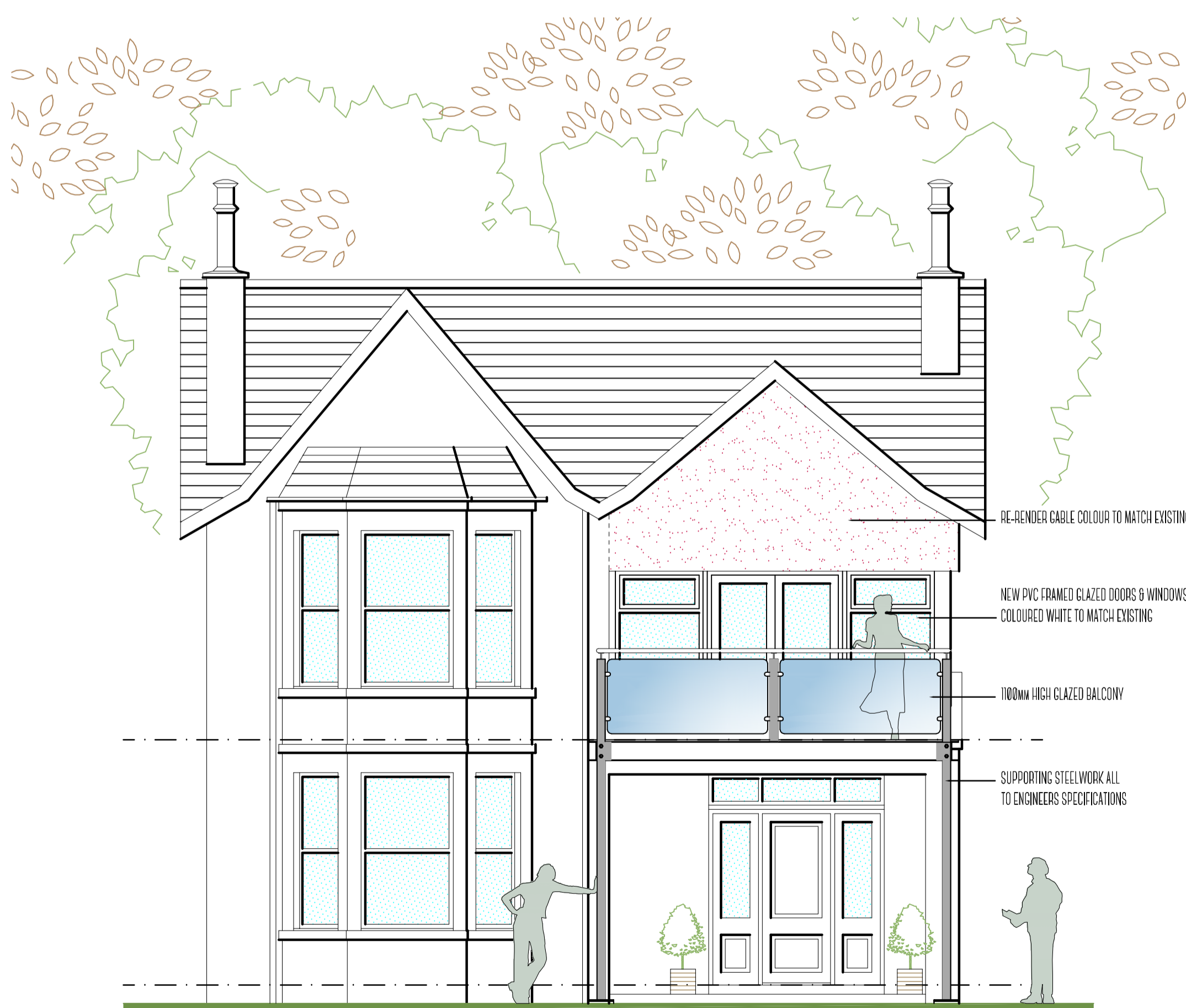
PROPOSED SOUTH ELEVATION SCALE 1:50 @ A1
