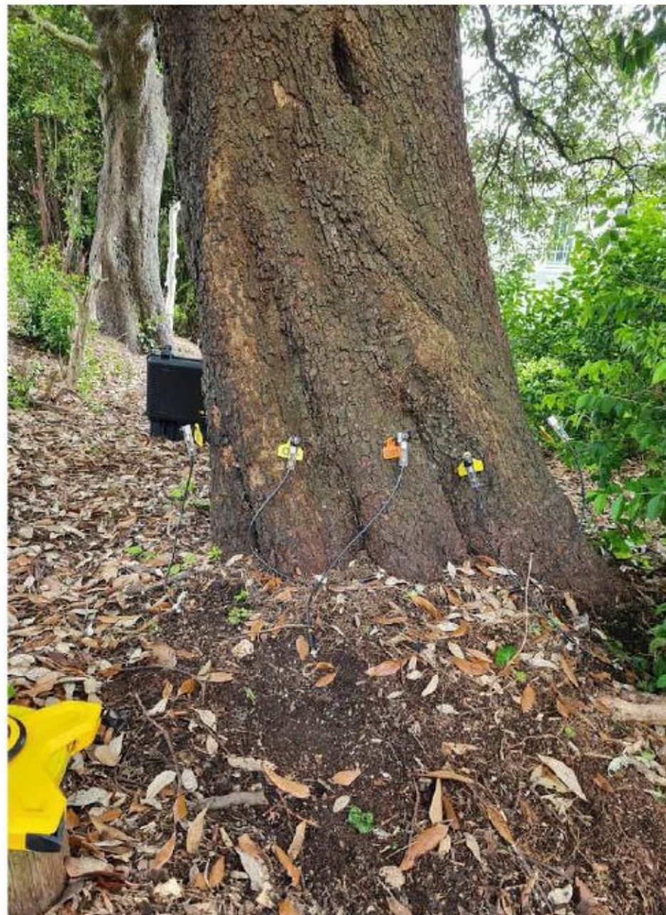
Arborsonic set up looking South ( sensors @300mm)
