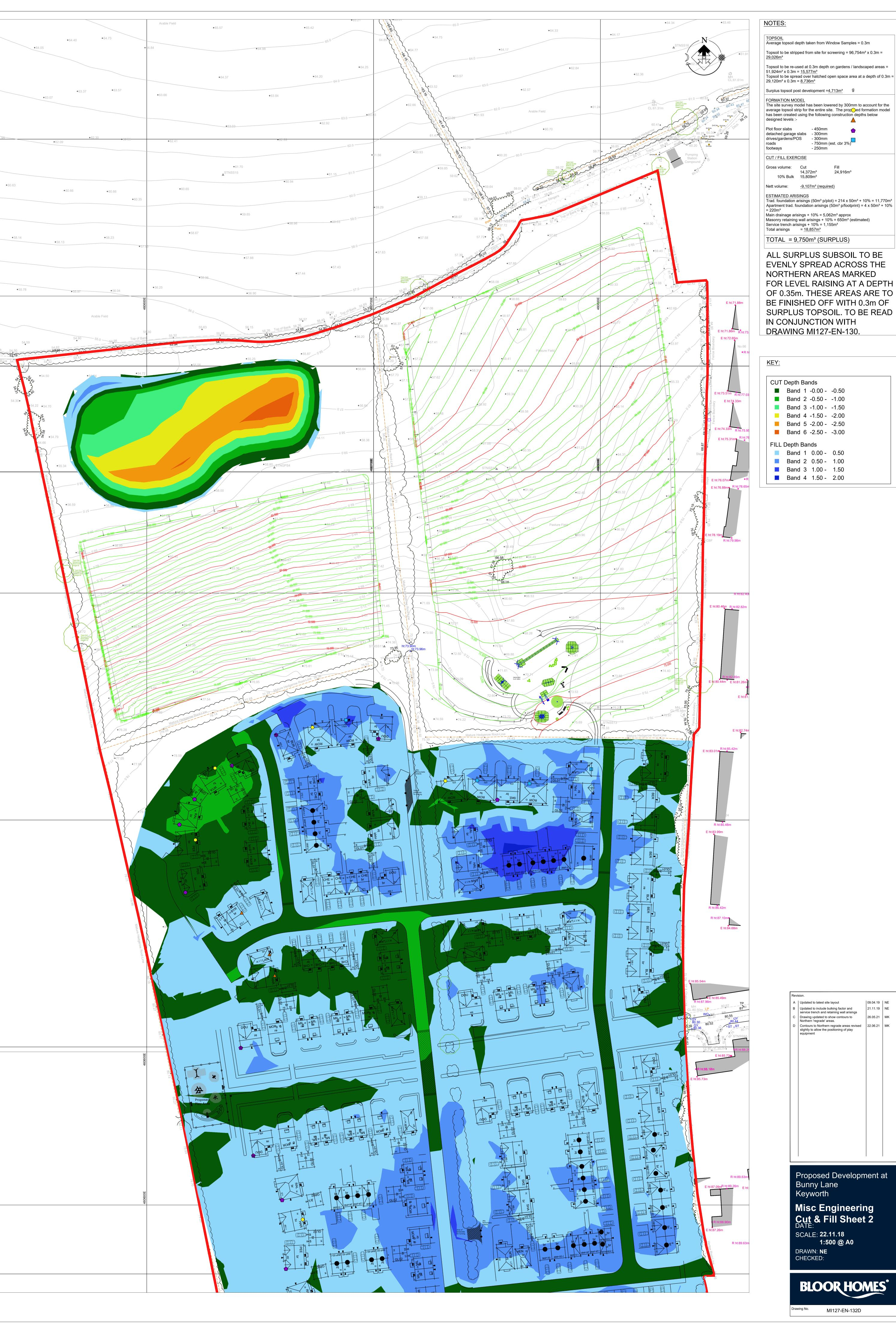
Topsoil to be re-used at 0.3m depth on gardens / landscaped areas =  $51,924\text{m}^2 \times 0.3\text{m} = \frac{15,577\text{m}^3}{15,577\text{m}^3}$ Topsoil to be spread over hatched open space area at a depth of 0.3m =  $29,120\text{m}^2 \times 0.3\text{m} = \frac{8,736\text{m}^3}{15,5730\text{m}^3}$ Surplus topsoil post development =4,713m³ 9 FORMATION MODEL
