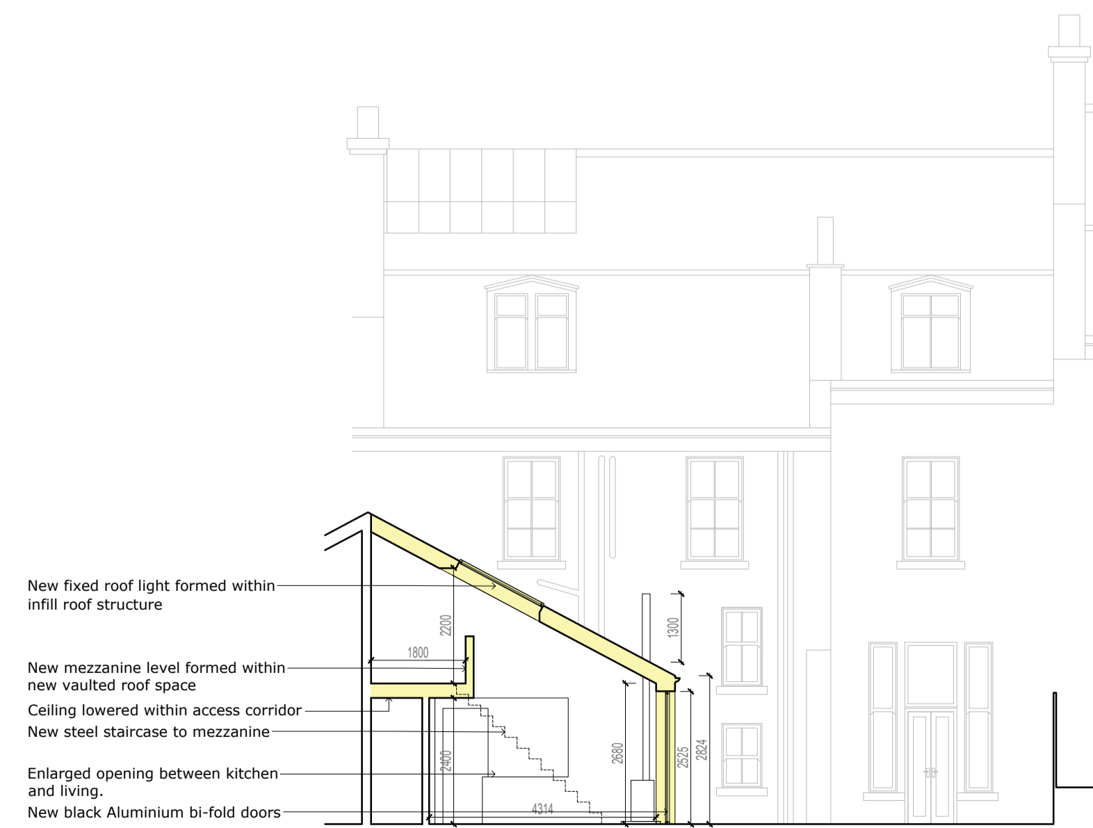
05 Section A-A - As Proposed 1:100 @ A1
