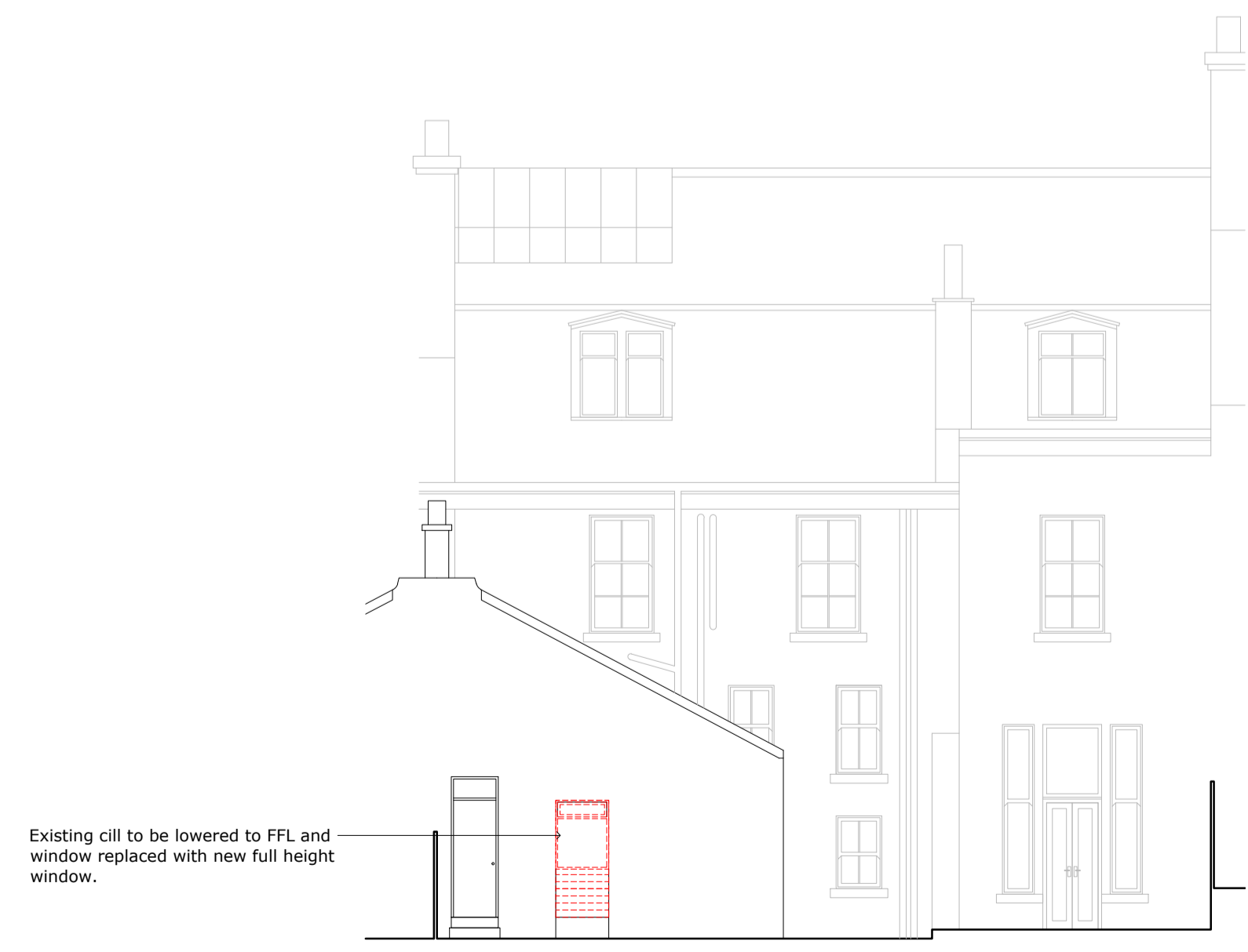
07 South East Elevation - As Existing 1:100 @ A1
