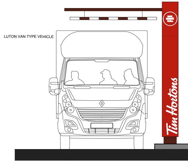
DTS 3A HEIGHT LIMITER 3.6m
