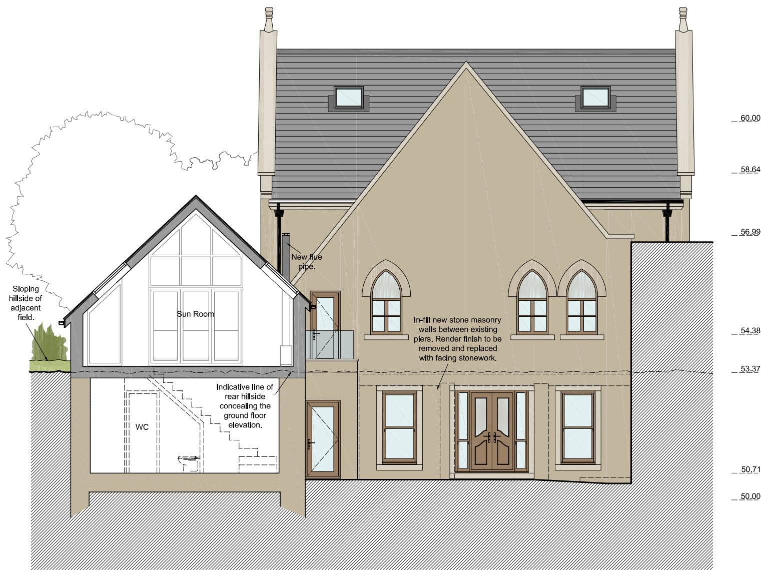
Proposed Rear Elevation (North-East) & Section A-A
