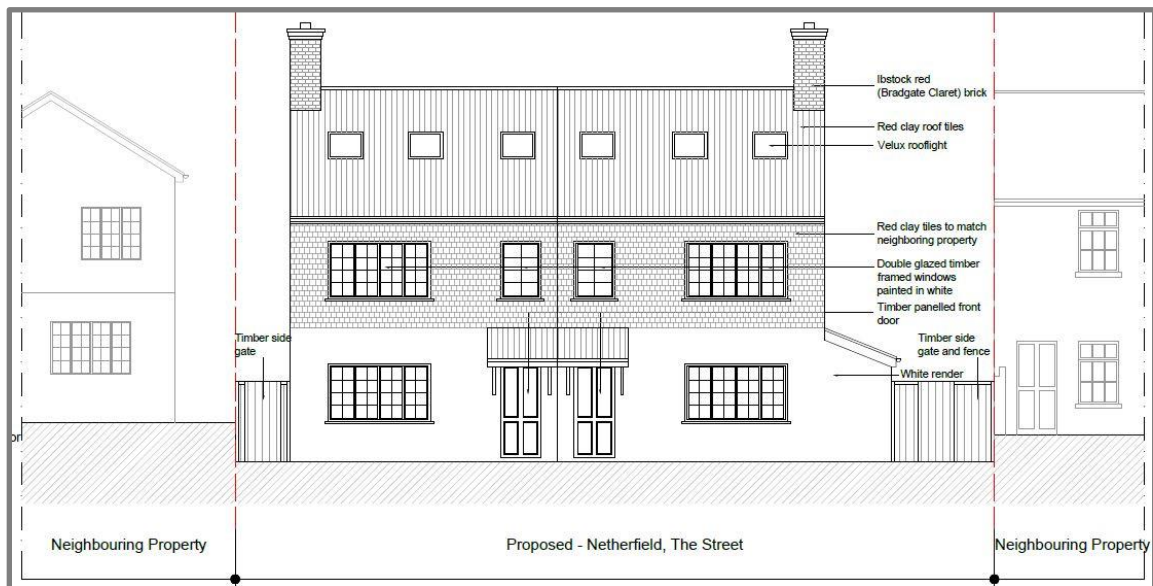
Fig. 5: Proposed Front Elevation
