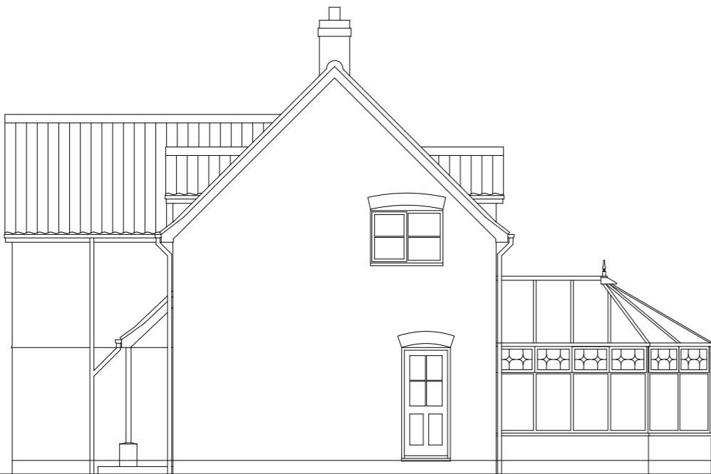
Existing East Elevation 1:100 @ A3
