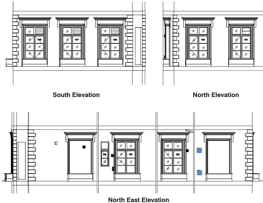
Existing external elevations showing proposed location of new vents and existing casement windows
