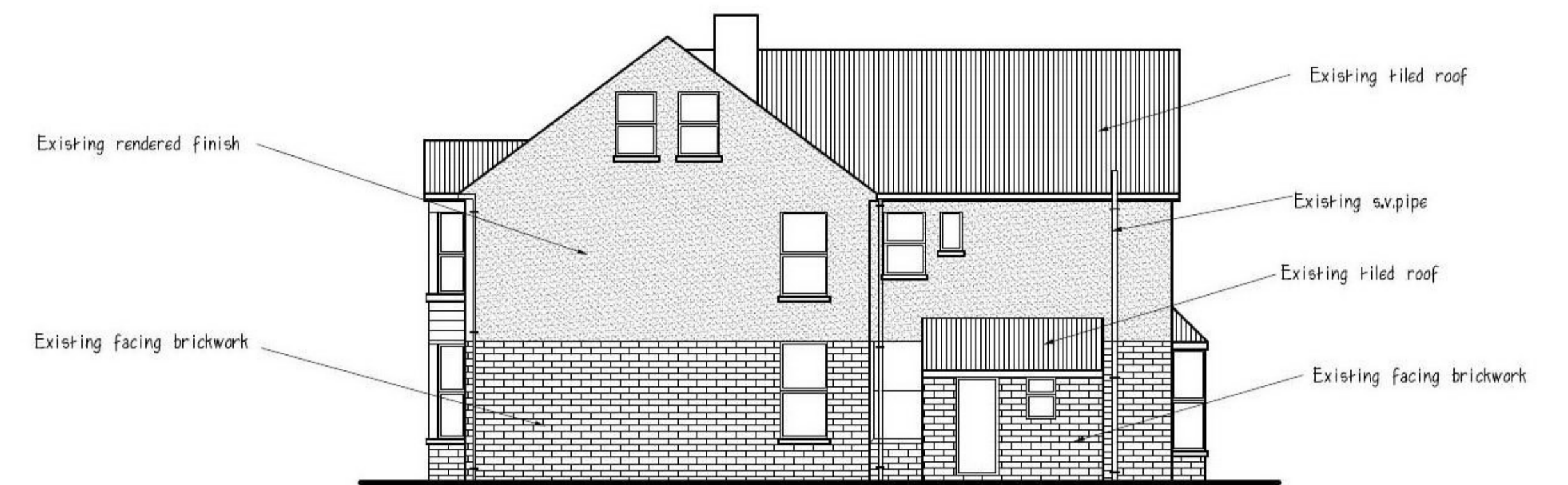
Existing side elevation
