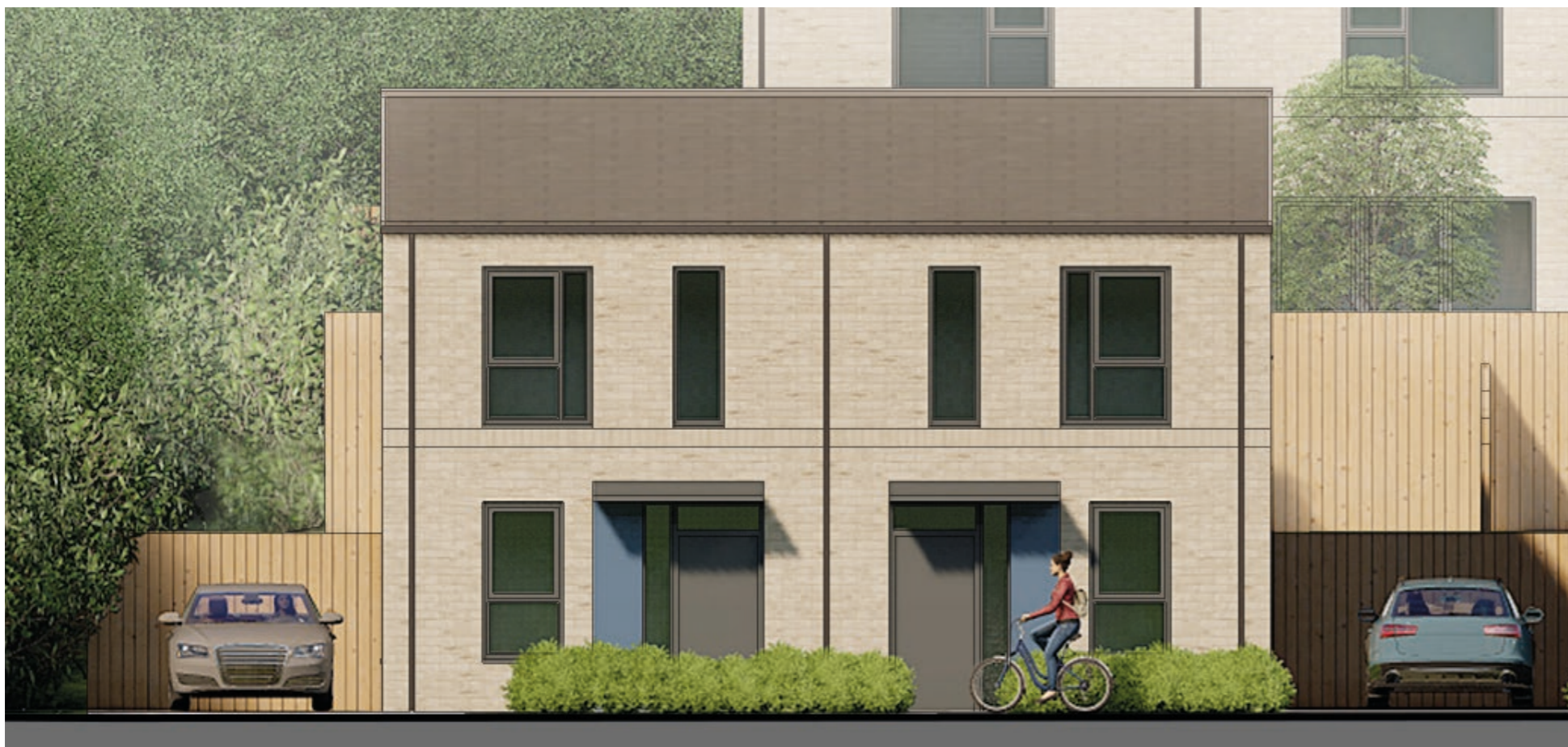
Street elevation showing plots 30 and 31. Buff multi facing brick with feature render panels to entrance doors.
